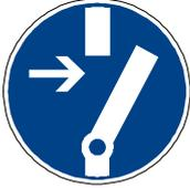
Only connect the product to current circuits that can be switched off by a switch (all poles disconnected). When working on the product, secure the system/machine in which the product is installed against switching on again.
